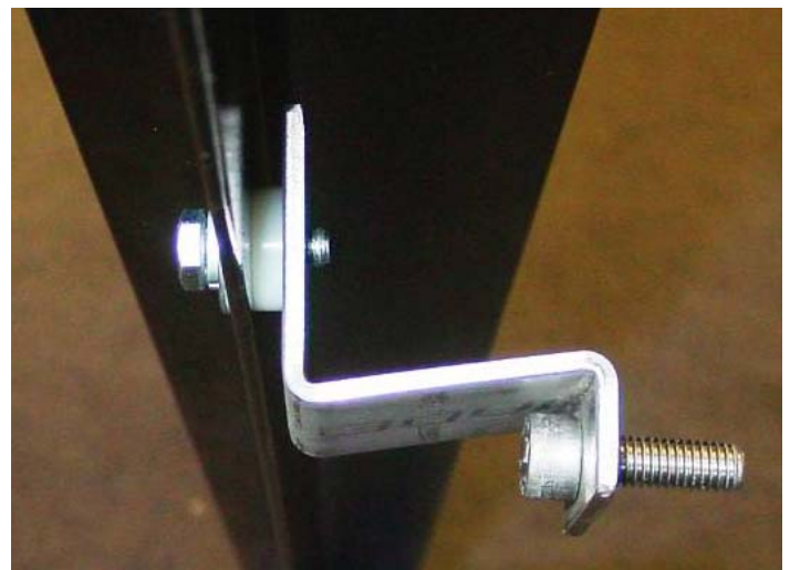
Bottom view of RETRAX rail with mounting hardware attached. (not mounted on truck)
